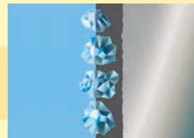
Diamond crystals in an electro-deposited metal bond.
